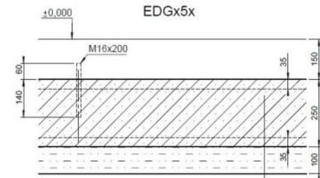
ZÁKL. DESKA / FOUNDATION BASEPLATE / FUNDAMENTPLATTE
