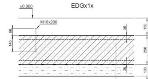
ZÁKL. DESKA / FOUNDATION BASEPLATE / FUNDAMENTPLATTE
